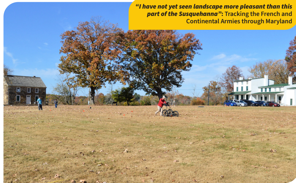
Figure 2. Ground penetrating radar survey at Elk Landing, Cecil County, Maryland (Courtesy of MHT 2024)
