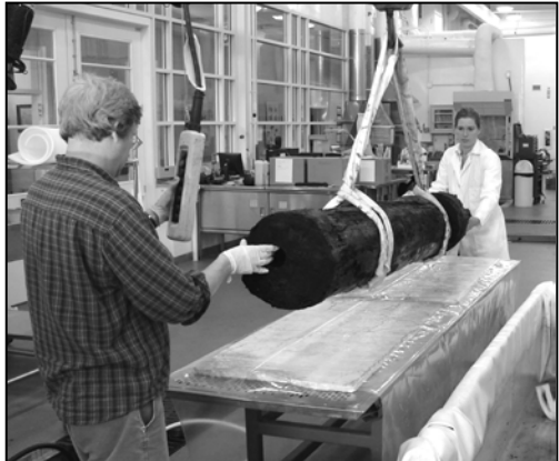
Conservators lifting oversized object from PEG tank.
