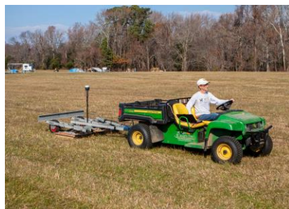
A multi-channel GPR system being towed across the Mill Field (Photo: HSMC).
