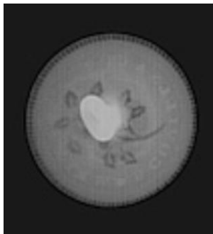
Figure 1: X-ray image of a 19 th -century button from HSMC's Town Center Site, showing details including the button's back shank, decorative border, filigree, and letters.
